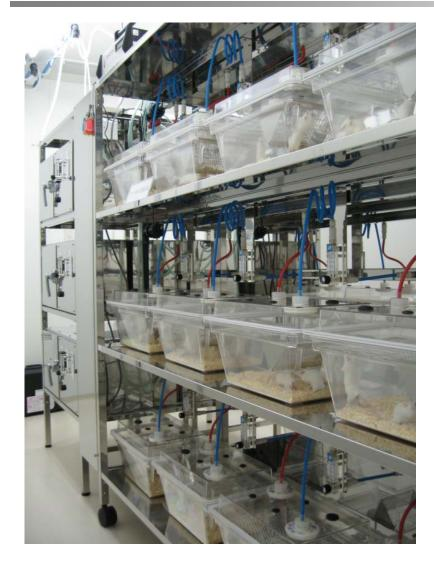
This is a facility developed for radon inhalation experiments with small animals, and is the first large-scale facility of its kind in Japan.
